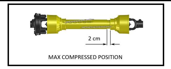
A driveshaft too long may cause structural damages to the tractor and machine. If the driveshaft is too long, it may be adapted by removing it and shortening the tubes according to the instructions provided by the Manufacturer in its use and maintenance manual.
