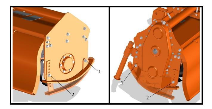
When finished, verify that both skids are at same level, and check if the front of the tiller is leveled to the back, when lowered to the ground. Adjust with the 3-point top link if necessary.
