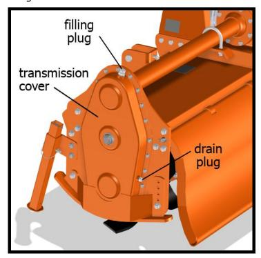
Check the oil level every 50 hours, making sure it reachs the level plug on the transmission cover. If the oil is below this level, fill up oil till restore the level.
